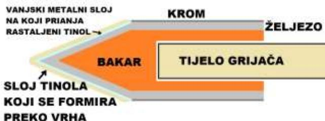
ILUSTRACIJA PRESJEKA VRHA S VIŠE SLOJEVA METALA
